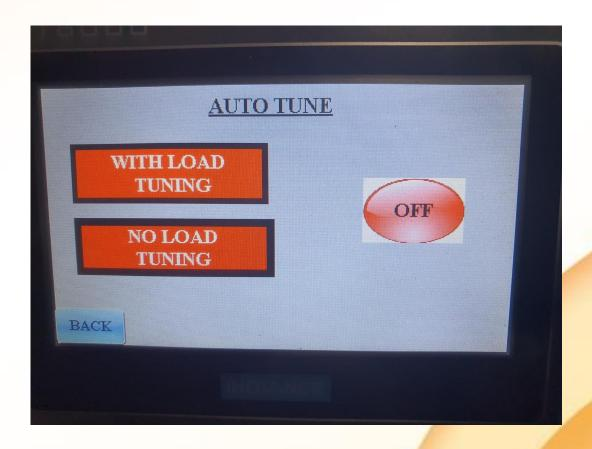
If the Controller is connected to the machine and you are doing the tuning, then it is called WITH LOAD TUNING. If the Controller is not connected to the machine, then it is called NO LOAD TUNING. You can do either one.
