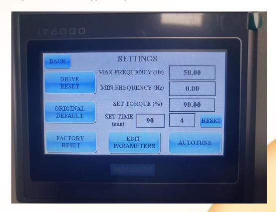
You do not have to set the Max Speed, Min Speed and Torque. Leave them at the original factory settings.
